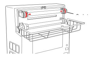
3 Pull out the terminals of the insect trap lamp along the grooves of the fluorescent lamp sockets.
