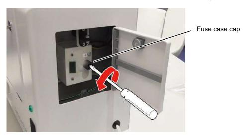
3 Remove the old fuse from the fuse case, and then install the new fuse.
