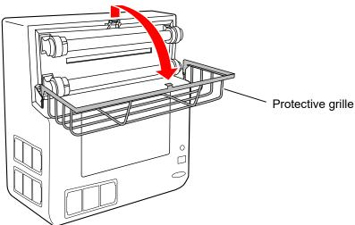
2 Rotate counterclockwise the left and right socket caps of the insect trap lamp to remove them.
