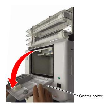
4 Strip the tape that has secured the insect trap bag fixing clip during shipment, and then remove the clip.
