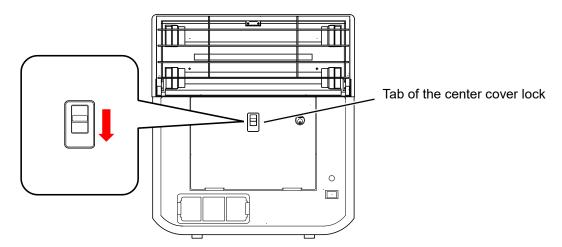
3 Open the center cover toward the front, and then remove the old attractant from the attractant pocket on the back of the center cover.
