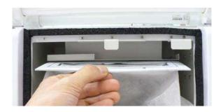
6 Fix the insect trap bag using the insect trap bag fixing clip.
