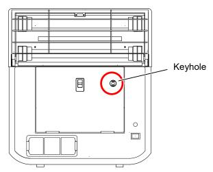
2 Lower the tab of the center cover lock to unlock the center cover.
