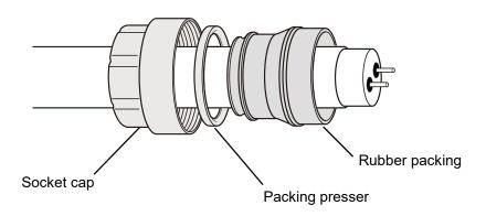
Insert the pins on both ends of the insect trap lamp into the grooves on the fluorescent lamp sockets. Push the insect trap lamp until you hear a click to mount it.
